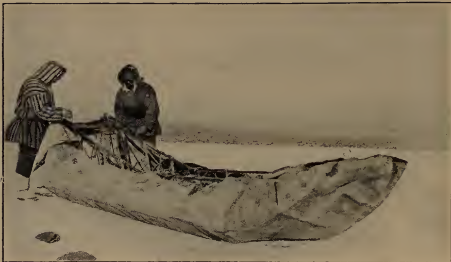
CONVERTING A SLED INTO A BOAT BY WRAPPING IT IN A TARPAULIN.
